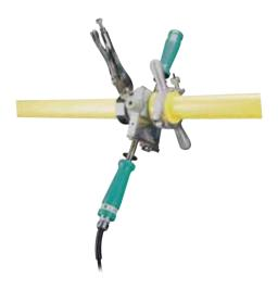
McElroy® Socket Tooling will fuse 1/2" CTS to 4" IPS (16mm to 125mm) pipe and is perfect for installing fittings. Select the heater, heater adapter, depth gauge/chamfer tool, and a cold ring tool for your specific application.
