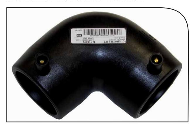
Electrofusion fittings incorporate an electrical heating wire. When activated for a specified period of time by an electrofusion processor, the surface of the pipe and the fitting melt together, thus creating one homogeneous pipe.
