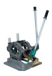
The McElroy® Pit Bull® 14 fuses 1" IPS to 4" DIPS (32mm to 110mm) pipe. It is a compact, lightweight, highly reliable, and rugged machine. The machine incorporates McElroy's patented Centerline Guidance System and is designed to butt fuse tees, ells, and other fittings with consistent, high-quality results. The machine's semi-automatic locking cam system maintains force during the cooling cycle.
