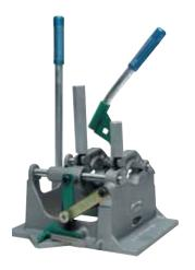
The 2LC will butt fuse 1/2" CTS to 2" IPS (16mm to 60mm) pipe. It employs a semi-automatic locking cam (LC) system to maintain force during the cooling cycle. The 2LC incorporates McElroy's patented Centerline Guidance System and is designed to butt fuse tees, ells, and other fittings.
