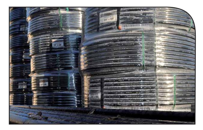
HDPE (high-density polyethylene) pipe is the preferred choice for geothermal heating and cooling systems. HDPE pipe is economical, durable, light weight, flexible, and weather resistant. In addition when properly fused, joints become as strong as or stronger than the pipe itself.
