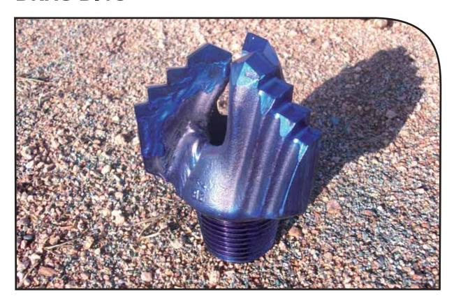
Hole Products offers a wide selection of Step and Chevron type drag bits for use in a variety of formations. Drag bits are offered with three or four wings in sizes ranging from 2 3/4" to 26".
