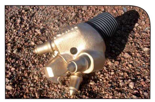
Claw bit are designed for drilling in soft to medium, unconsolidated formations including gravels, sandstone, and shales. They feature field replaceable bullet shaped cutters. Cutters are designed to rotate in their blocks to provide a self sharpening effect, thus extending the life of the bit.
