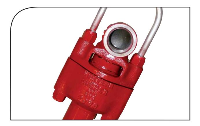
Hole Products offers a variety of quality top feed water swivels for use on conventional rotary drill rigs. Swivels are designed to provide a watertight rotating joint to connect the pump and drill string with a high pressure hose. Water swivels help pump water or other drilling fluids to the bottom of the bore hole.
