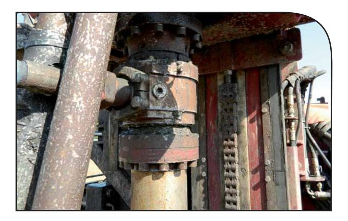
Hole Products offers a variety of quality side inlet water swivels, designed for use with hydraulic, top-head drive rigs and/or to convert auger rigs to circulating, rotary drilling rigs. Swivels are designed to provide a watertight rotating joint to connect the pump and drill string with a high pressure hose. Water swivels help pump water or other drilling fluids to the bottom of the bore hole.
