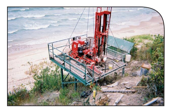
Augers and their associated tooling are used in several drilling markets including geotechnical, environmental, exploration, and construction. Augers are recognized as versatile and effective tools for advancing the borehole, and therefore are the preferred drilling method for a variety of applications.
